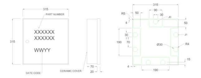
Figure 1 Module Outline and Markings; Units in mils
